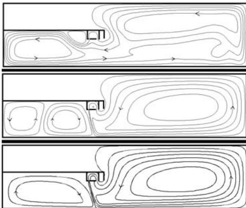
Figure 5. Streamline patterns (kg/s) for the 3 regimes: natural convection, mixed convection and forced convection. Simulations of geometry B.
