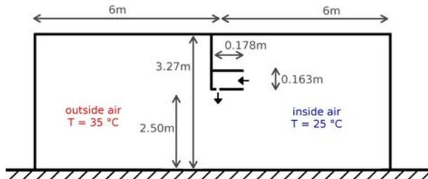
Figure 3. CFD geometry A, also used by Costa [9].
