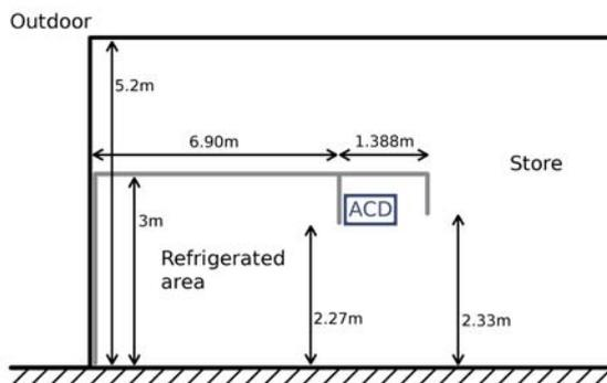
Figure 1. Geometrical properties of the test site
