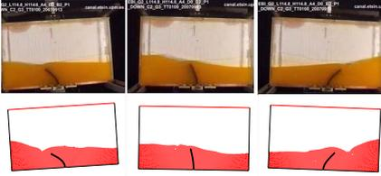
Figure 2. Snapshots (after 1.84 s, 2.12 s and 2.56 s) from experiments and simulations of the flexible baffle in a rolling tank.
