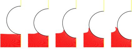
Figure 1. Snapshots (every 10 ms) of the impact of a composite cylinder on a water surface.
