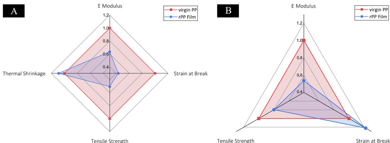
**Fig. 4.** Mechanical performance comparison between recovered rPP Films and virgin PP on biaxially oriented (A) and cast (B) films.
