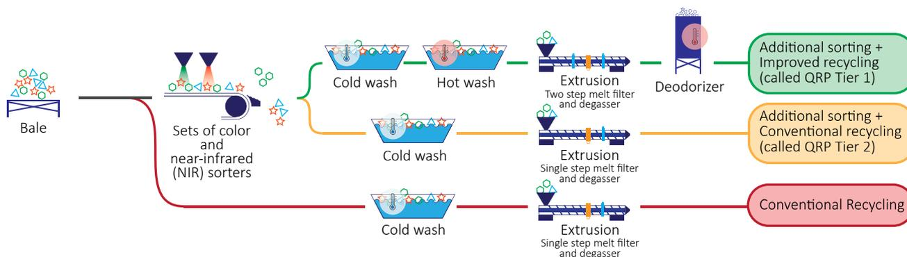
Fig. 1. Scheme of a current conventional mechanical recycling process (bottom), which can be expanded either with only additional sorting (middle) or replaced entirely by additional sorting and improved recycling (top).
