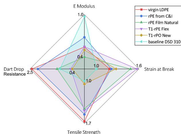
Fig. 3. Mechanical performance comparison between recovered regranulates, baseline and reference materials on blown films. Axes are scaled differently for ease of visual interpretation.
