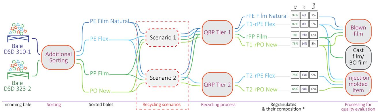
Fig. 2. Flow of materials within different steps of QRP at two scenarios and the composition of the regranulates (\*= compositional data are taken from Lase et al., (2022)). Cast film and biaxially oriented (BO) film samples are produced and provided by external partners.
