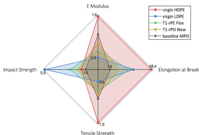
Fig. 5. Mechanical performance comparison between T1-rPE Flex and T1-rPO New regranulates and baseline and reference materials on injection molded specimens.
