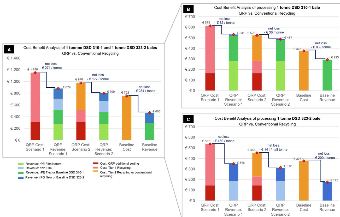
Fig. 6. Net profit/loss of the QRP scenario 1, QRP scenario 2, and baseline scenario: (A) processing 1 tonne DSD 310–1 and 1 tonne DSD 323–2 bales, (B) processing 1 tonne DSD 310–1 bale, and (C) processing 1 tonne DSD 323–2 bale.
