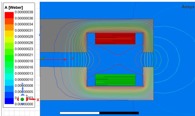
**Fig. 6 (b)** An EE cores inductor with thicker copper of the two parallel windings
