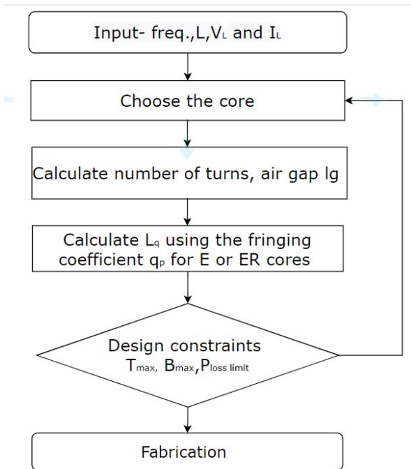
**Fig. 2** Analytical design flowchart for planar flat wire inductors.
