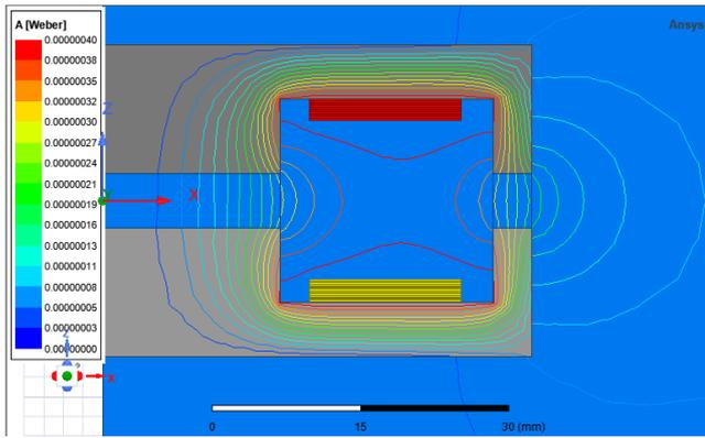
**Fig.6 (a)** Ansys Multiphysics FEM model of gapped inductors - axisymmetric representation, an EE cores inductor with two parallel windings
