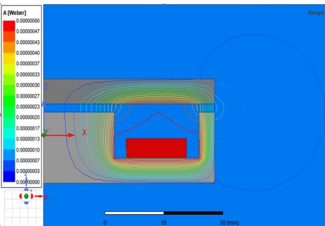
**Fig.6 (c)** An EI cores inductor with one winding
