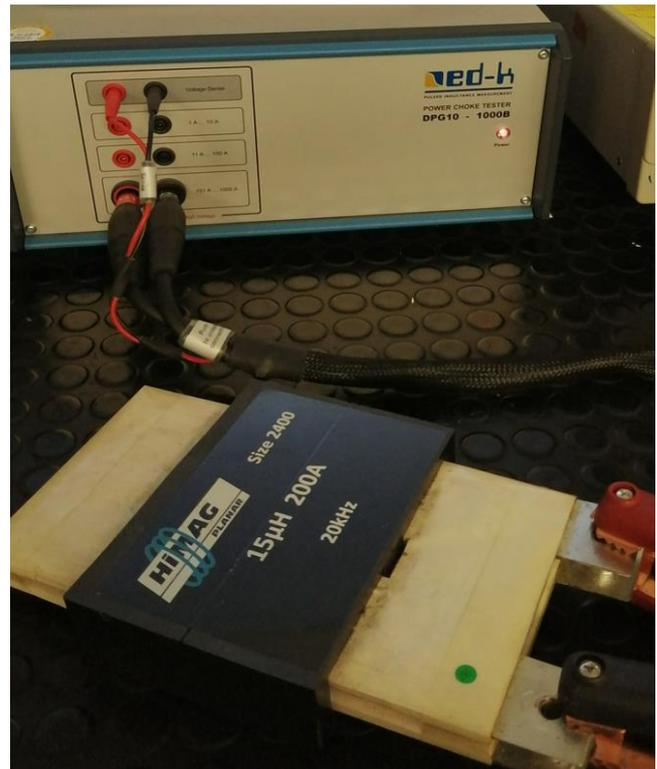
Fig.9 Setup for the 15uH inductor test measurement with Ed-k choke tester.
