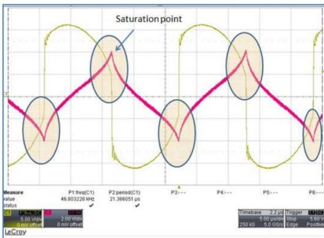
Fig.8 Experimental waveforms (a) Output voltage and current (b) Output voltage, current and saturation points.
