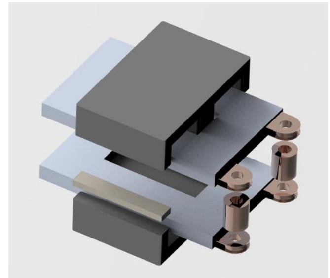
**Fig. 5** Planar inductor structure with two parallel windings.
