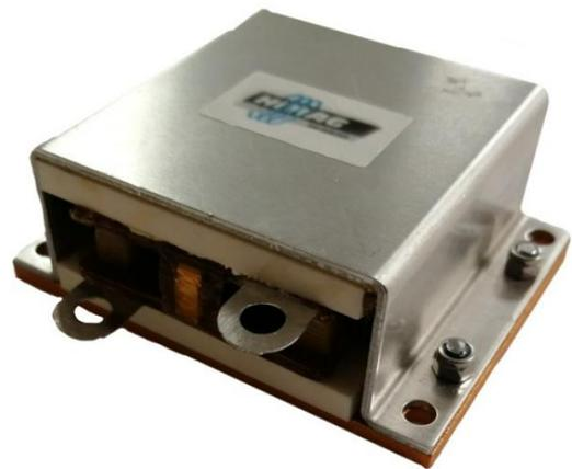
**Fig.7(a)** Prototypes of the inductors with flat wire;- A planar inductor with flat copper and ceramic blocks.
