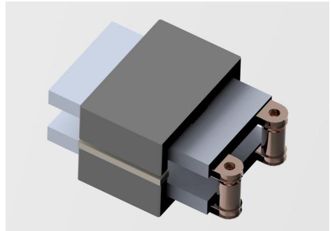
**Fig. 4** Planar inductor with EE cores.
