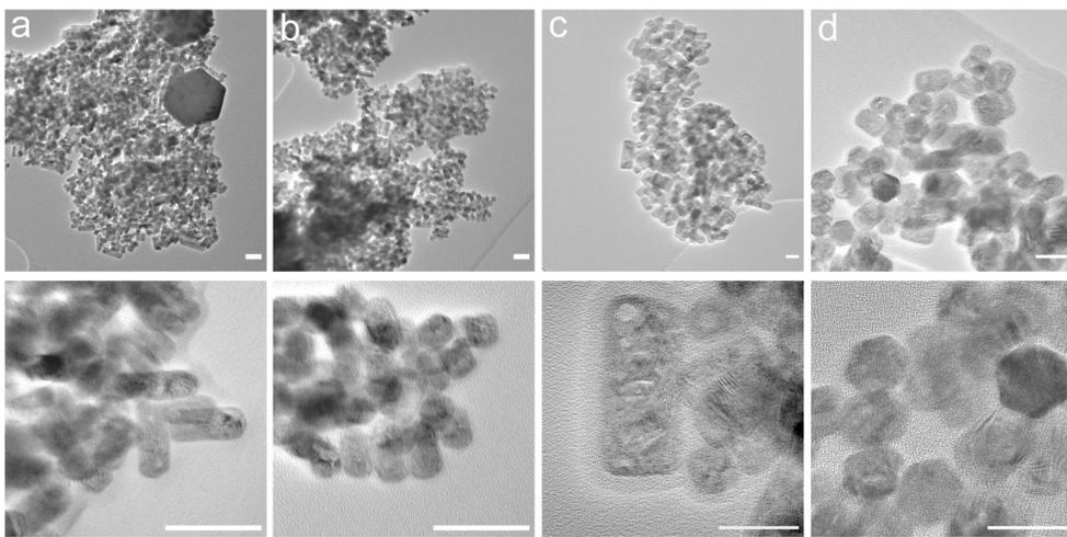
Fig. 1 TEM images of 2%Er,18%Yb:LaF<sub>3</sub> synthesized with 2.5 mmol NaOH (a) or 2 mmol NaF (b). (c) shows the 2%Er,18%Yb,2%Tm:LaF<sub>3</sub> synthesized with 2.5 mmol NaOH and (d) the respective sample synthesized with 2 mmol NaF. An overview is shown in the top row, a close-up in the bottom row. The scale bar is 50 nm for all images.
