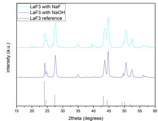
Fig. 2 PXRD patterns of 2%Er,18%Yb:LaF<sub>3</sub> synthesized with 2.5 mmol NaOH and 2 mmol NaF compared to the ICSD ID 23972 reference data for LaF<sub>3</sub>.
