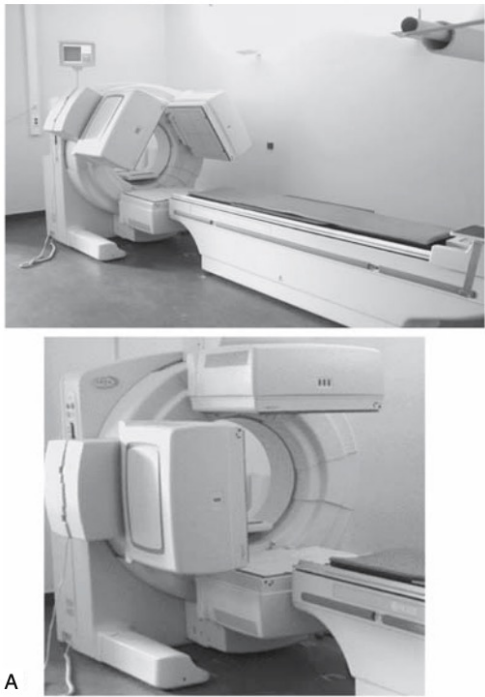
Figure 10.1. A: A three-head gamma camera-based positron emission tomography (GCPET) system (Philips Irix 3000). The three heads can be placed at different gantry angles with respect to each other and can be used for both routine SPECT as well as for coincidence imaging. B: A schematic representation of the coincidence circuit used in a GCPET system. For a coincidence event to be detected, the two photons must be detected within the 15-ns timing window and should lie within the specified energy range.
