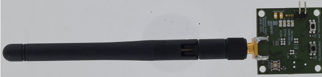
Fig. 5: The soldered PCB with the hinged dual-band Delta 7A from Siretta connected.
