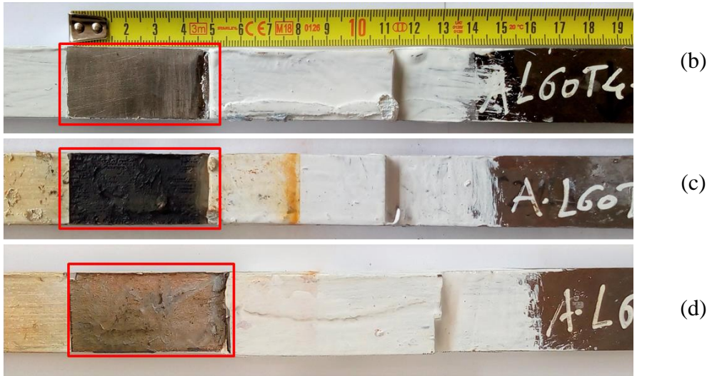
Figure 3 Electrochemical cells (a) and DLJ specimens: (b) unaged, (c) after 24 hours of ageing, (d) after an additional 6 hours of environmental exposure.
