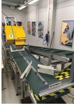
Fig. 1: A physical infrastructure part of the testbed with a LIBS equipment installed and material circulating on the conveyor
