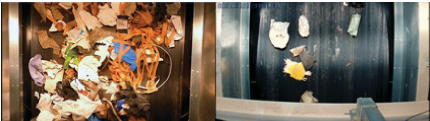
Fig. 7: Photo impressions of object singling on the 2D (left) and 3D (right) line
