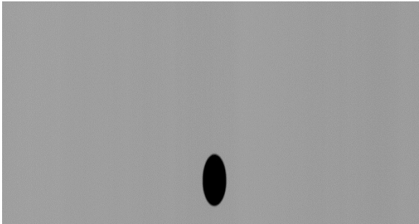
Fig. 5: Cropped image of the line scan camera showing a falling ball. The line scan frequency is higher as it should to get quadratic pixels, therefore the object looks elliptic.
