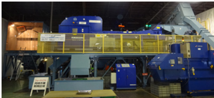
Fig. 6: Pilot plant to realize horizontal recycling for aluminium in the NEDO project (2010-2012)
