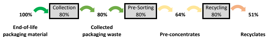
Fig. 1: Relevance of collection-, pre-sorting and recycling-performance (80% exemplary performance) for the overall achieved recycling performance
