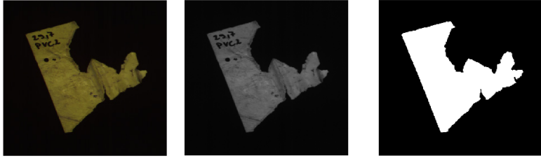
Fig. 1: Example of the used images: original RGB image (left), greyscale image (middle), and binary image (right) of singlified waste particle (Kandlbauer et al. 2021)
