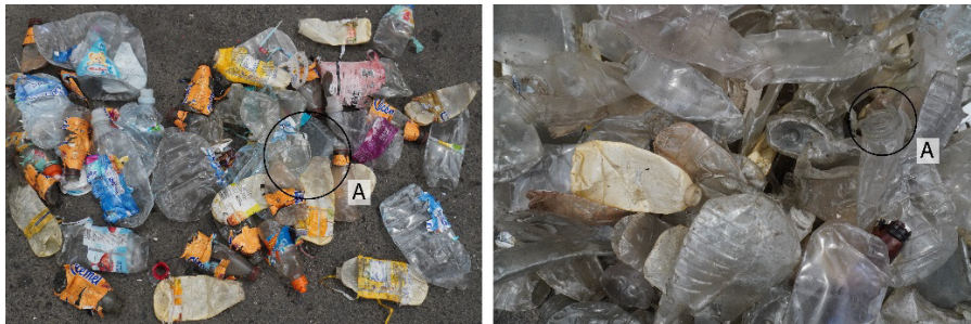
Fig. 7: Pictures of manually sorted “Partly delabelled” (left) and “No label” (right) material after delabelling. A: Exemplary bottles without caps.
