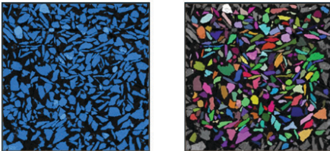
Fig. 5: Particle segmentation (a) and particle separation and rejection of particle touching the border (b)
