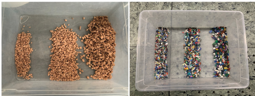
Fig. 2: Three particle size classifications (0 mm — 4.0 mm, 4.0 mm — 5.4 mm, and 5.4 mm — 10.0 mm) for the materials CDW (left) and plastic flakes (right)
