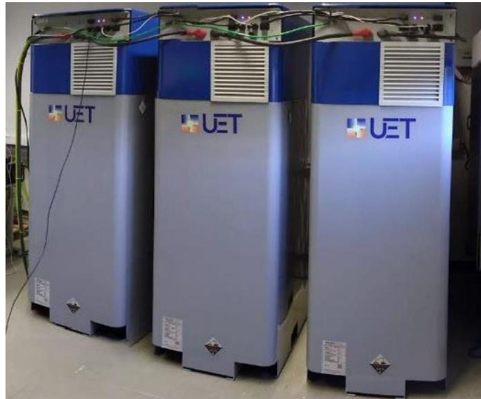
Figure 3. Series RFB test setup. Three UET RFBs are connected in series and form a string of batteries, which facilitates operation at greater voltages. The series setup has a nominal voltage of 144V and a maximum voltage of 192V.
