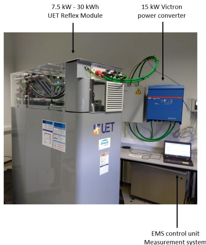
Figure 2. Single RFB test setup. The battery is controlled by an energy management system in a computer, which also handles communication between the inverter (blue box) and the battery. Aside from this, the computer also collects measurements via the battery management system, which is located at the top of the RFB module.
