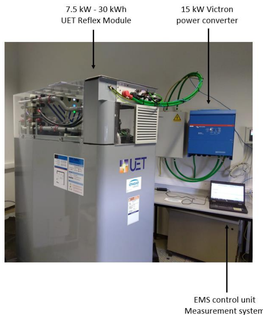
Figure 2. Single RFB test setup. The battery is controlled by an energy management system in a computer, which also handles communication between the inverter (blue box) and the battery. Aside from this, the computer also collects measurements via the battery management system, which is located at the top of the RFB module.
