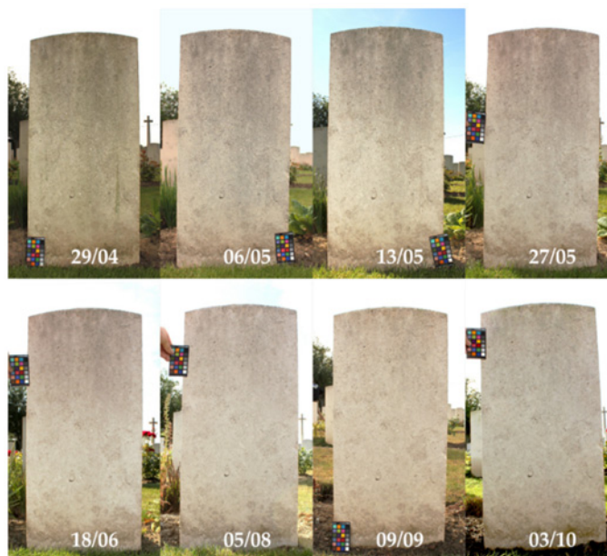
Figure 7. Evolution of grey-black biofilm in streaks and green biofilm (Site B).
