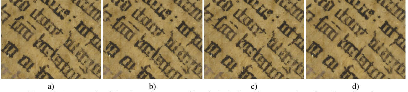
Figure 4: An example of the edge coherence problem in the independent processing of small patches of a large image. a,b,c) An example of removing cracks, provided that each subsequent processing begins with a shift of 0, 9 and 18 pixels, respectively, d) The result of combining all the images into one using the median filter.
