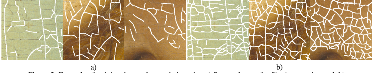
Figure 5: Example of training dataset for crack detection: a) Source dataset for Singing angels panel, b) Extended dataset for Singing angels panel
