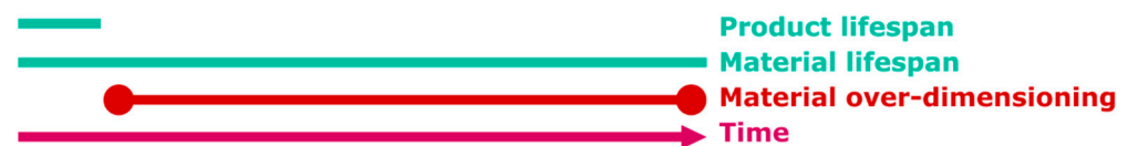
Figure 1. Time-in-use versus material lifespan, often resulting in a mismatch and so a material over-dimensioning.
