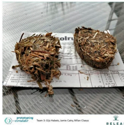
Figure 9. Example of students having some great success in their experiments with agar-agar binder material. Photo and quoted text by the students; Jamie Catry, Milan Claeys and Gijs Habets of the team "Natural fibers".
