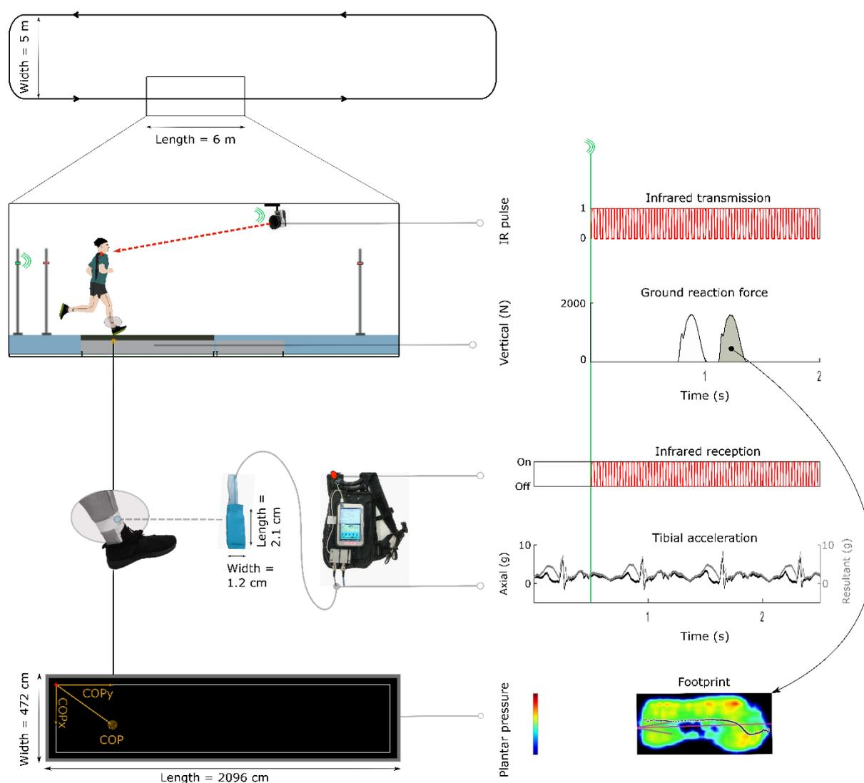
Figure 1. Schematic representation of the set-up in the laboratory: running course, measurement zone, measurement instruments and signals.
