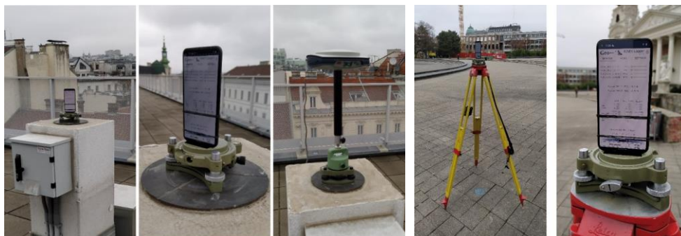
Figure 2. Smartphone und reference receiver SP80 on two neighbouring measuring pillars on the roof of the EI building of TU Wien and mobile measuring set-up on Karlsplatz.
