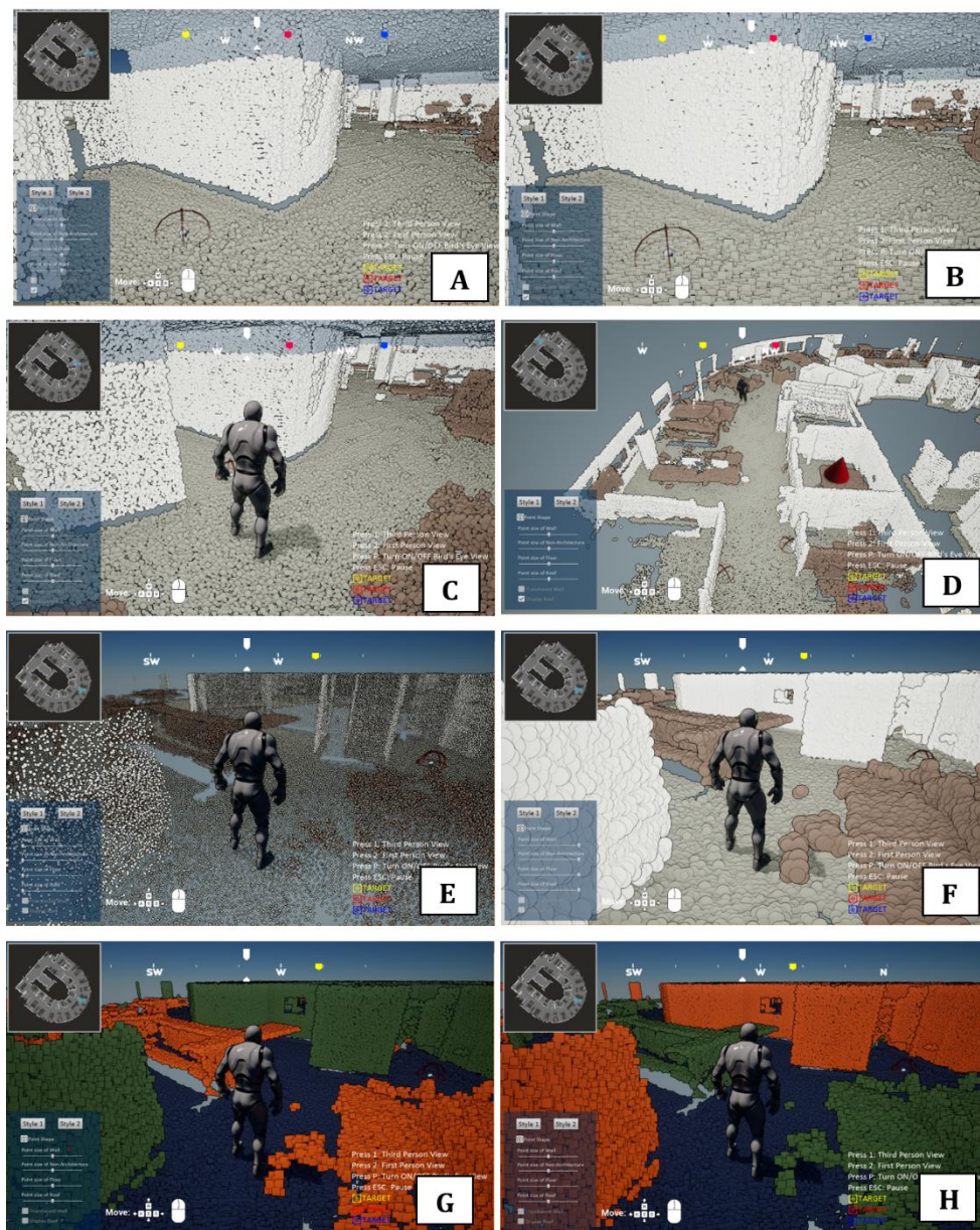
Figure 18. Visualization results: (A) circle points (first-person view), (B) square points (first-person view), (C) third-person view, (D) bird's eye view, (E) the smallest size points, (F) the biggest size points, (G) darker style 1, and (H) darker style 2
