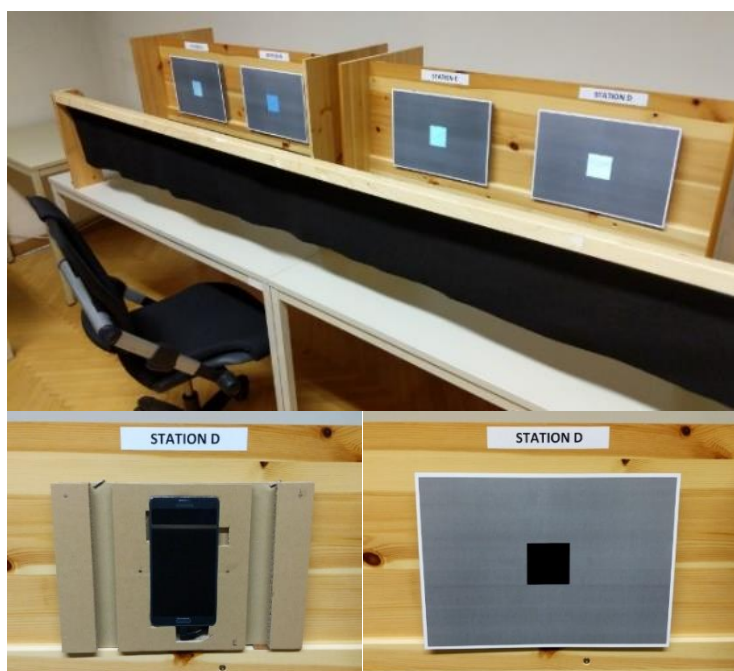
Figure 1. Lab setup for the study. Top: viewing stations with mobile phones of varying pixel densities mounted behind bezels, rail to ensure constant viewing distance, curtain to minimize reflections. Bottom left: mobile phone mounting fixture. Bottom right: Bezel covering mounting fixture to reveal an area of identical size for each station.
