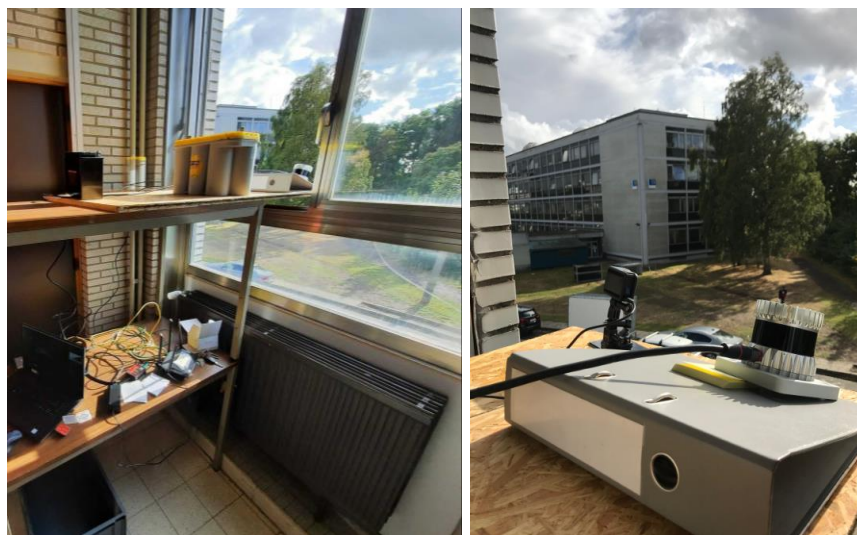
Figure 1. HPOI method laser scan set-up of case study at Ghent university campus (Belgium)
