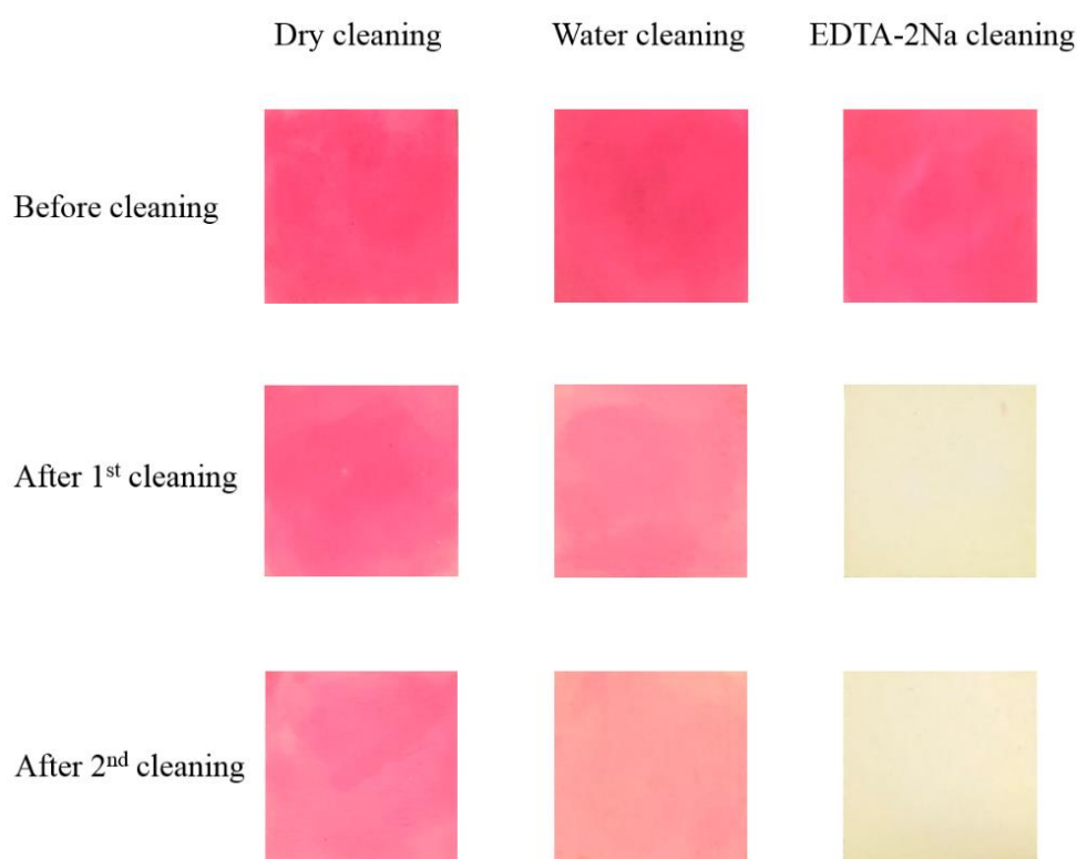
Fig. 2. Tests of the ability to remove lead ions from lab surface. Water cleaning has a better ability than dry cleaning, but the Pb 2+ still has the obvious residual. Only EDTA-2Na solution can completely remove Pb 2+ from the lab surface.
