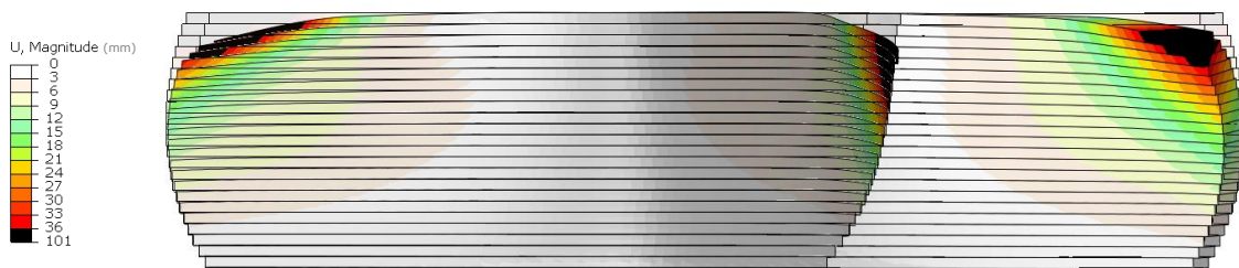
Figure 6. Deformations from CobraPrint : Material 202 at 22 layers
