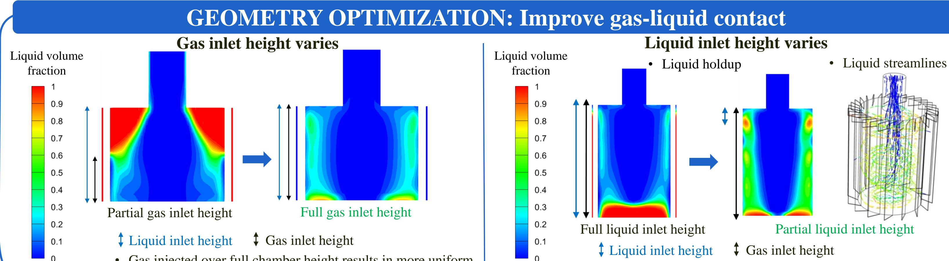
• Gas injected over full chamber height results in more uniform gas-liquid dispersion
