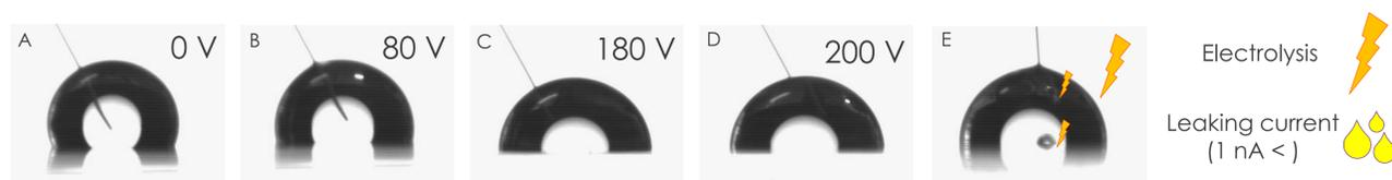
EWOD on SU-8-AlOx-FDTS stack upon 0, 80, 180 and 200 V application (A-D). Contact angle saturation is shown (C, D). Formation of air bubbles due to electrolysis on a SiNx-AlOx-FDTS dielectric stack at 140 V (E). On the right side, a legend with symbols representing electrolysis and leaking current is provided.
