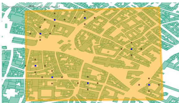
Figure 1: Considered portion of RAN of the city centre of Ghent (Belgium), composed by 8 macro cell BSs, each supported by 4 micro cell BSs.
