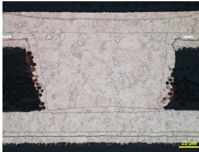
Figure 5. Etched microsection of a microvia after thermal cycling (200 cycles from -60 °C to +140 °C)
