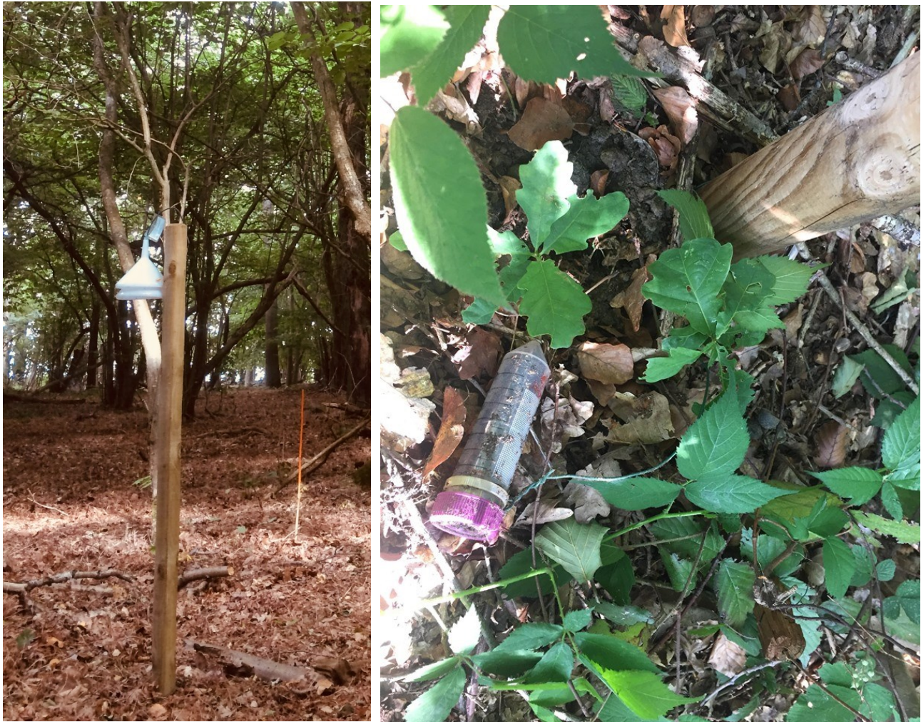
885 886 Figure A1: Set-up of the temperature sensors. Left: pole with radiation sheet, covering the air temperature data logger. Right: soil 887 logger protected by a plastic tube (here at the surface, normally buried at a depth of 5 cm).
