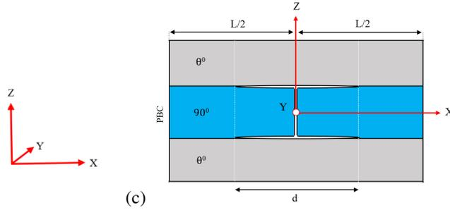
**Figure 1.** Schematic demonstration of different idealized damage scenarios in a  $[\theta/90_{0.5}]_s$  laminate; (a) ply cracking, (b) delamination and (c) ply cracks and delamination.
