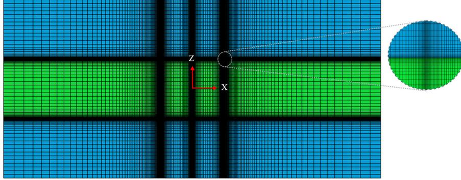
**Figure 2.** Finite element mesh details of composite laminate including ply cracks and local delamination.
