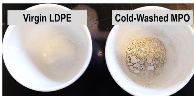
**Figure 1.** Inorganics remaining after heating ~4 g of ground sample to 600 °C in the muffle furnace
