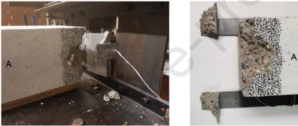
Figure 7. Debonding in the concrete prism for specimens A1, A2 and A3
