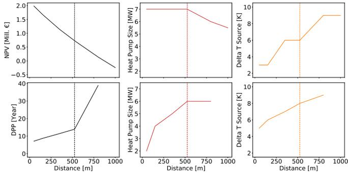
Figure 6. Sensitivity on distance between heat source and sink.
