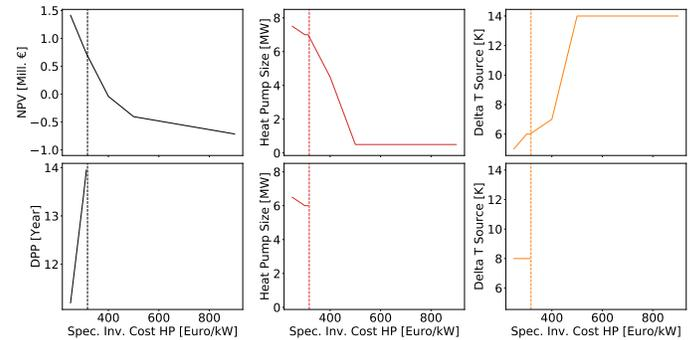
**Figure 5.** Sensitivity of the heat pump investment cost on the optimum parameters.
