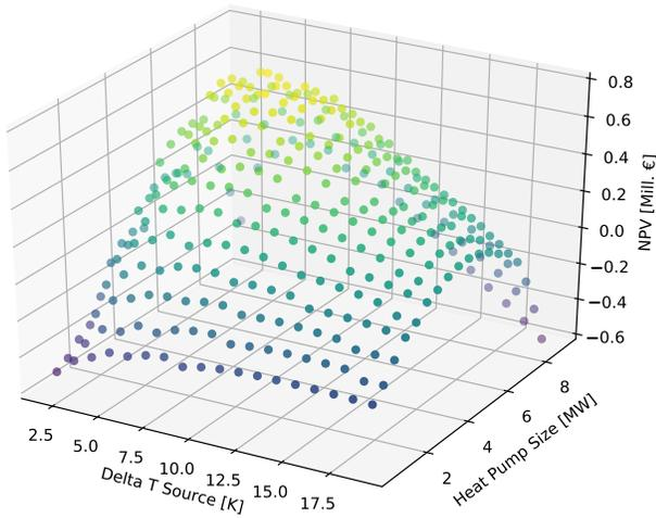
**Figure 3.** NPV in function of heat source temperature glide and heat pump size.
