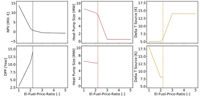
Figure 7. Sensitivity on electricity cost to fuel price ratio.
