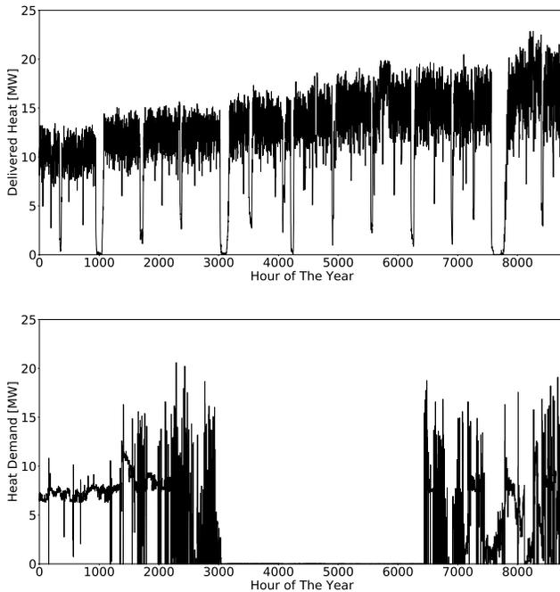
**Figure 2.** Heat load profiles of the cooling loop and the hall heating.
