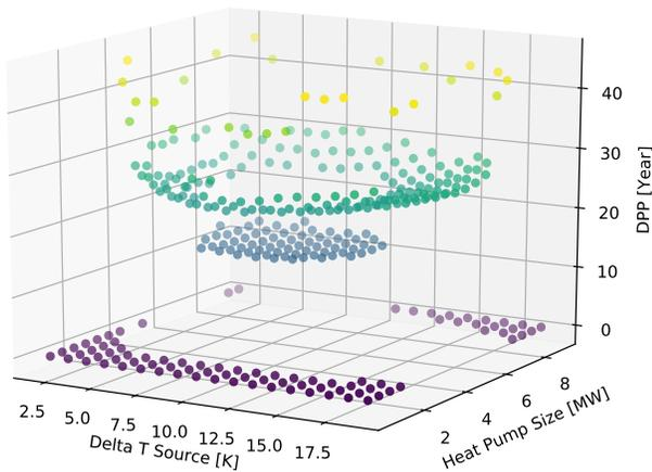
**Figure 4.** DPP in function of heat source temperature glide and heat pump size.
