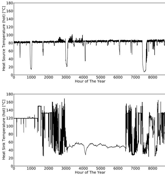
**Figure 1.** Temperature profiles of the cooling loop return temperature and hall heating supply temperature.
