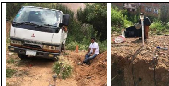
Fig. 3. Left: the vehicle tyres pass the more closely to the Jet Fill tensiometers installed. Right: BC 302 load cells were inserted horizontally near Jet Fill tensiometers; the pit wall is far enough away from the zone of influence of the tyre.
