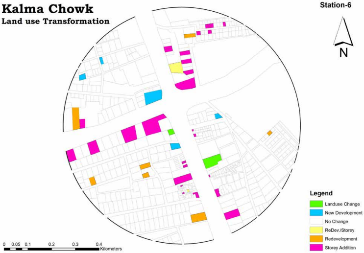
Figure 65 Land-use transformation at Kalma Chowk station
