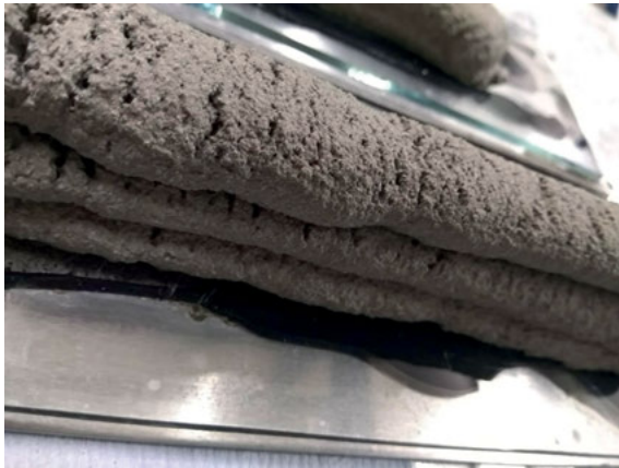
Figure 5.1: Three-dimensional printing of cementitious materials with SAPs by continuous layering.
