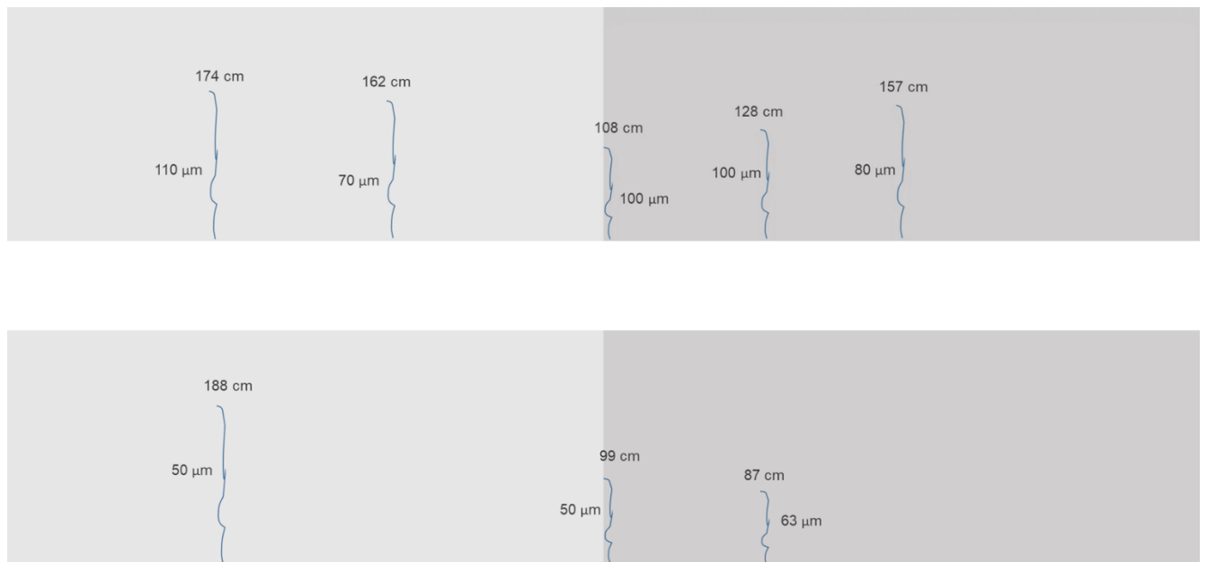
Figure 13 - Cracking pattern of wall REF1, showing the total height of the crack measured from the bottom [cm] and the average width [ \mu\text{m} ]. The upper part of the figure represents the side A and the bottom part of the figure represents the side B of the wall. The darker grey area had been treated with external curing agent.
