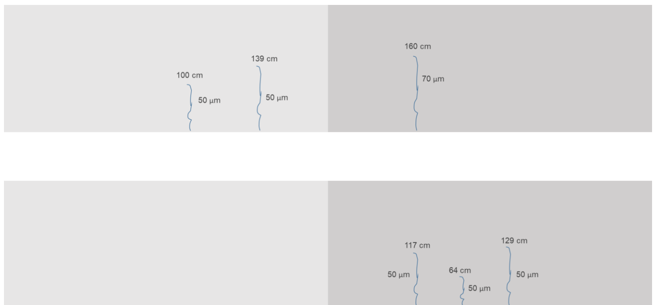
Figure 14 - Cracking pattern of wall REF2, showing the total height of the crack measured from the bottom [cm] and the average width [ \mu\text{m} ]. The upper part of the figure represents the side A and the bottom part of the figure represents the side B of the wall. The darker grey area had been treated with external curing agent.
