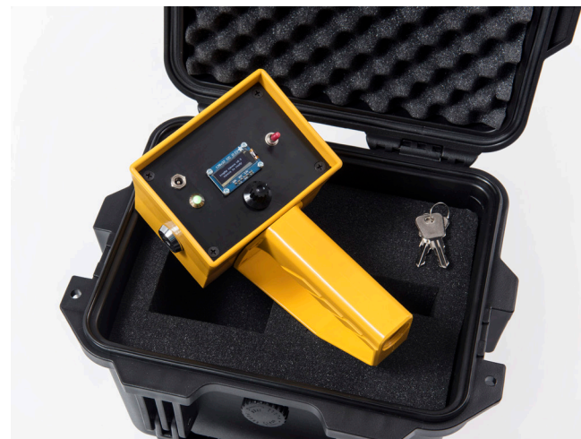
Trophy Camera v0.9 , 2017, Raspberry Pi Zero W, Full HD camera module for RaspberryPi, 5000mAh powerbank, monochrome 128 x 32 SPI OLED graphic display, plastic casing, 115 x 85 x 191 mm © Dries Depoorter and Max Pinckers. Permanent collection FOMU Antwerp, Belgium
