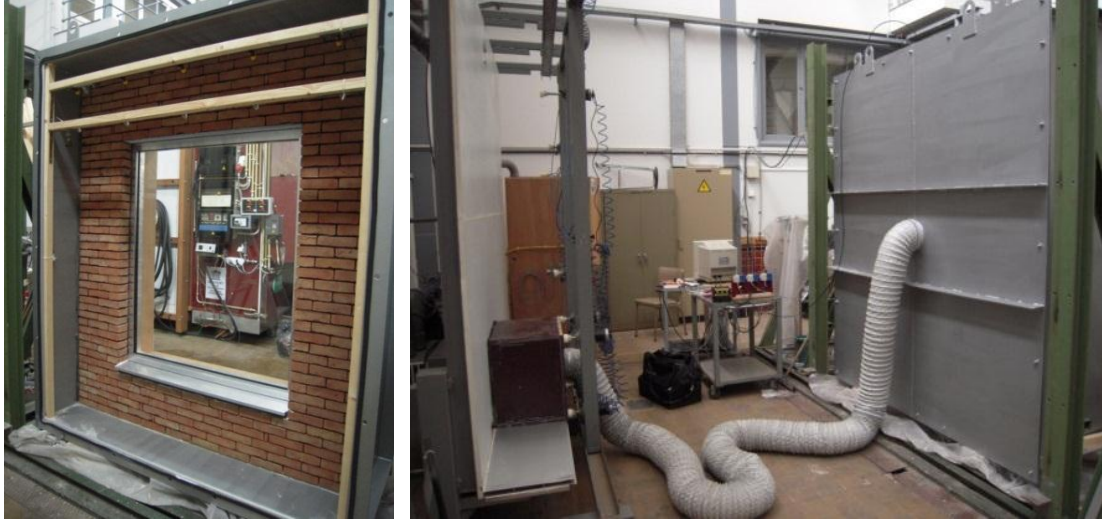
Figure 5: Left: Spray racks installed in front of the brick cavity wall specimens according to EN 12865 [18]; Right: Test specimen connected to test rig with flexible tube
