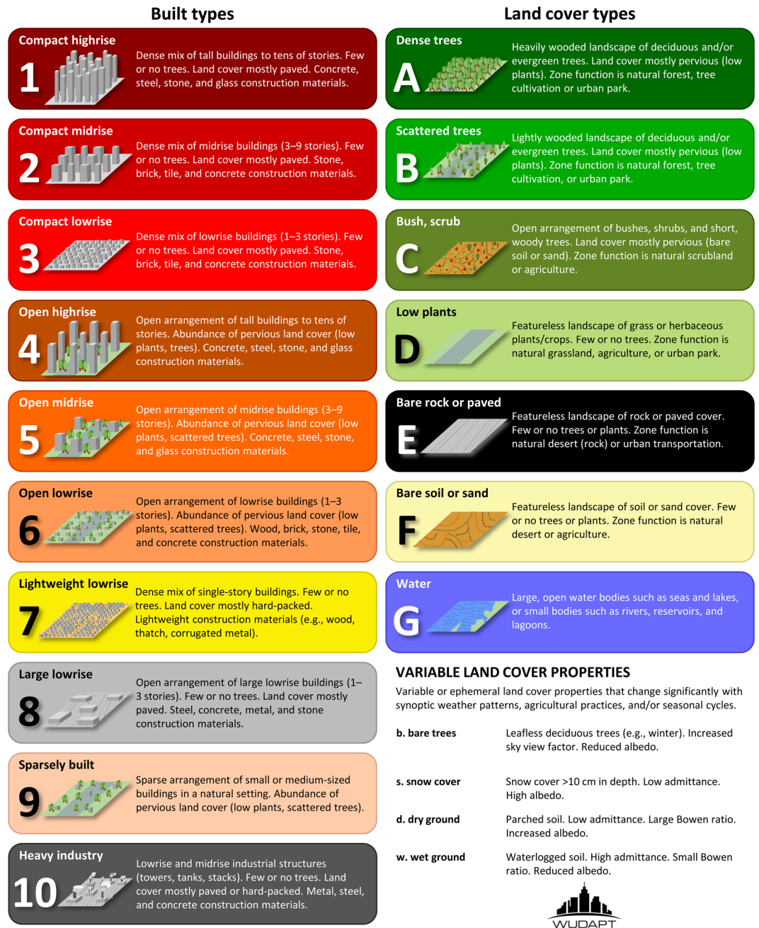
Fig. 1 Urban (1–10) and natural (A–G) Local Climate Zone definitions (adapted from Table 2 in Stewart and Oke 27 , default LCZ colors according to Bechtel et al. 31 ).
