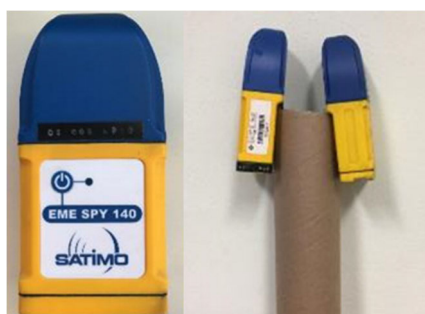
FIGURE 4. Personal exposimeters EME SPY 140 (Satimo) attached to a cardboard tube ready to carry out the measurements.
