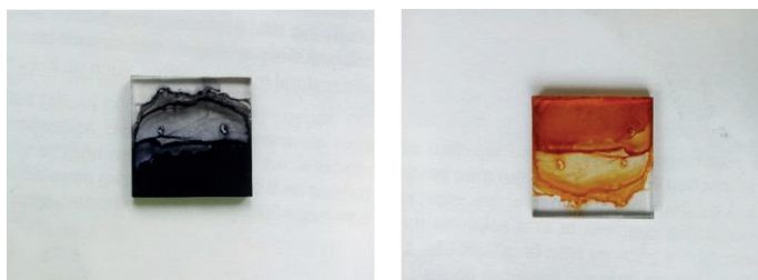
Figure S6.34. The photocatalyst-coated FTO substrate before (left) and after (right) soaking in ethanol.
