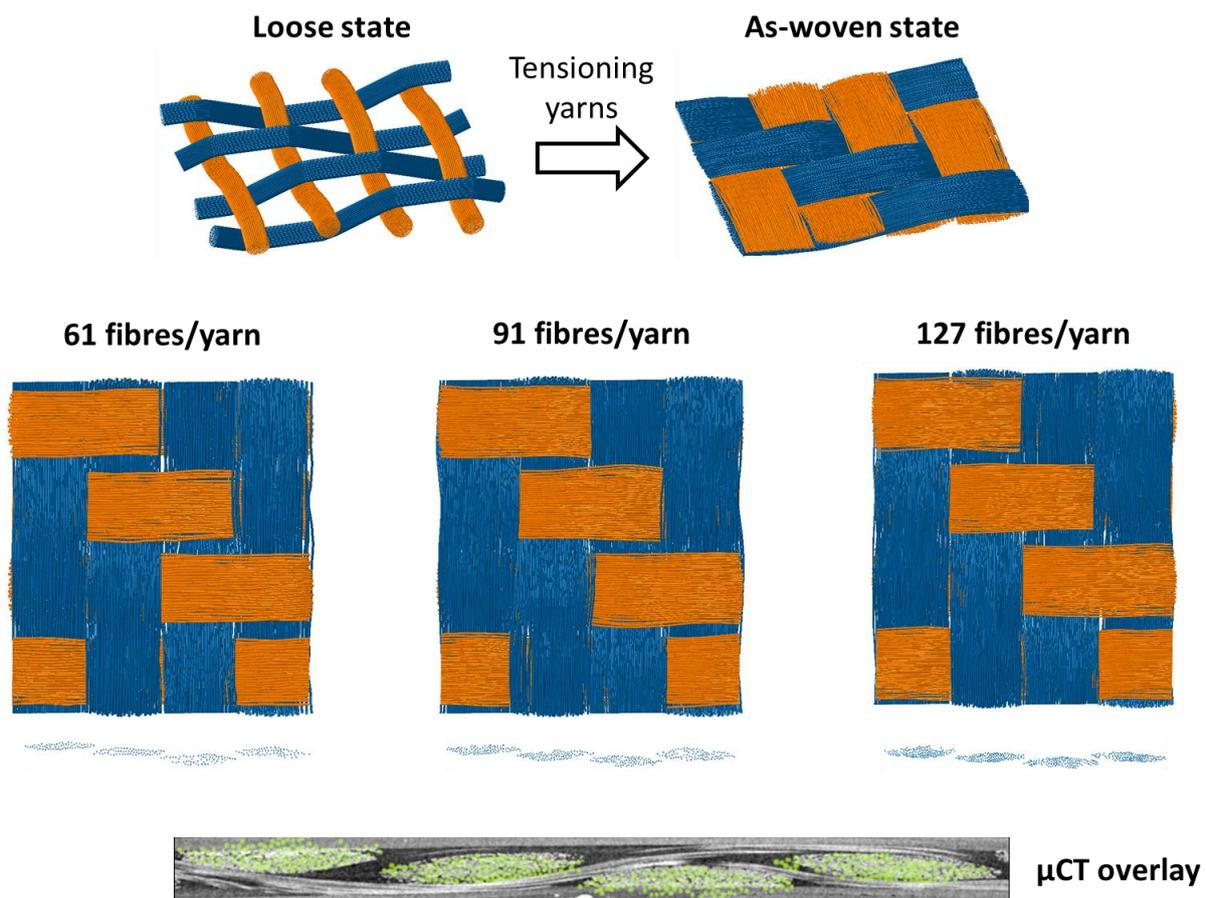
**Figure 3** - The as-woven state of the fabric is modelled based on the tensioning of an idealized fabric (here a 2x2 twill weave). The results for different amounts of virtual fibers per yarn show that discretization into 61 fibers/yarn suffices to predict the overall as-woven geometry.
