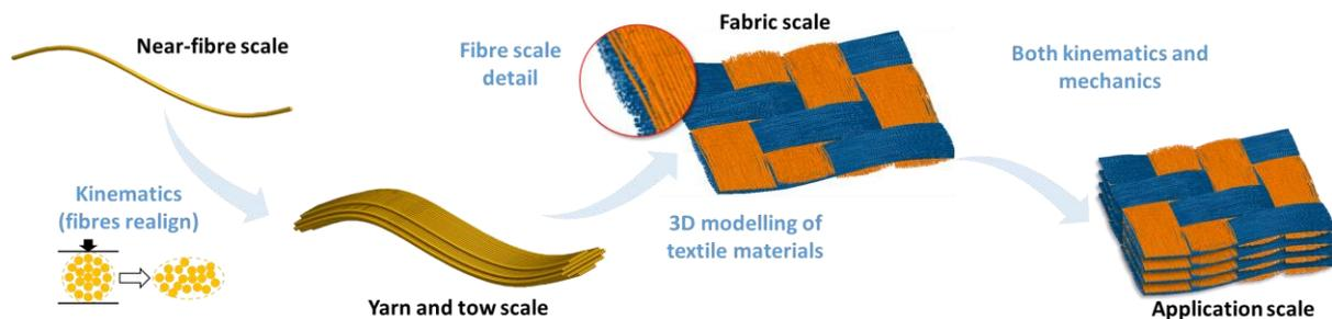
**Figure 1** - Concept of the virtual fiber approach, from yarn/tow scale to fabric scale to application scale. Yarns and tows are discretized into a discrete number of virtual fibers. This way, there is no need for complex constitutive material models, rather, the fibrous behavior of the textile is implemented in a natural manner.
