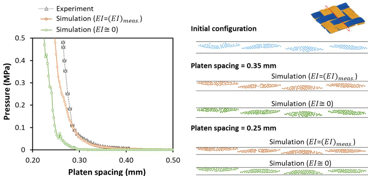
**Figure 6** - Compressive response of fabric simulated with and without bending stiffness of the virtual fibers show that while kinematically similar (yarn cross-sections are visualized on the right-hand side), the mechanical response (left-hand side) is better predicted when bending stiffness is considered.
