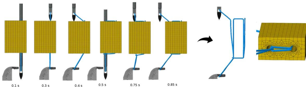
**Figure 4** - Yarn behavior and final yarn path in the stitching of a foam panel.
