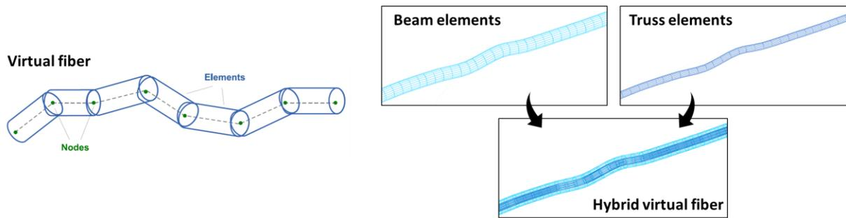
**Figure 2** - A virtual fiber consist of a chain of truss- and/or beam-like elements.
