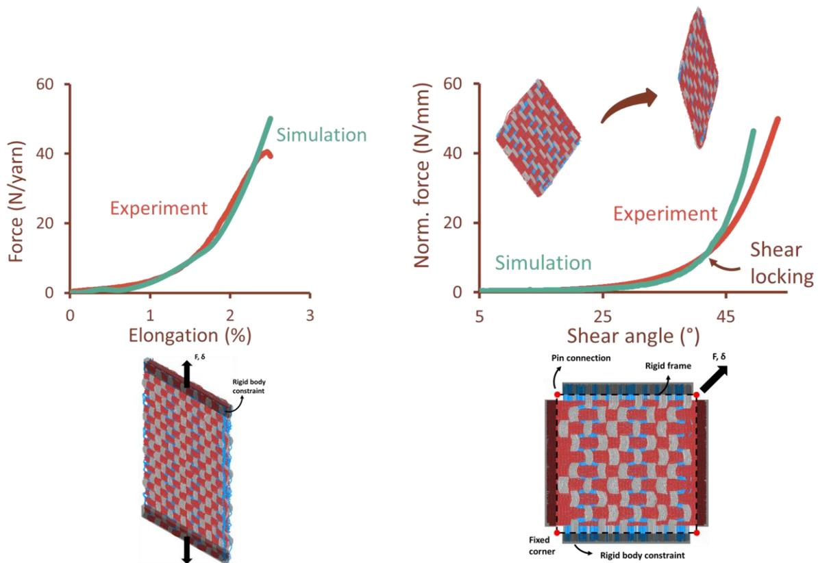
**Figure 5** - Tensile test simulation and the resulting force versus elongation diagram (left). Picture frame simulation and the resulting force versus shear angle diagram (right).
