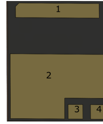
Fig. 7. (GS66508B) Package:(1) Drain, (2) Source, (3) Gate, (4) Source sense
