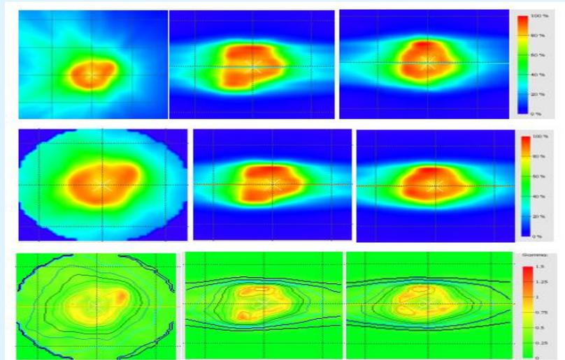
**Figure 2:** A screenshot from Octavius 4D measurements analyzed in Verisoft. Showing the result of 3 beams SBRT delivery of lung cases. Panels (a), (b), and (c) show dose map in eclipse, Octavius calculated dose matrices and g-distribution in transversal, sagittal and coronal plans column wise respectively having 3 beams of SBRT delivery for lung case.
