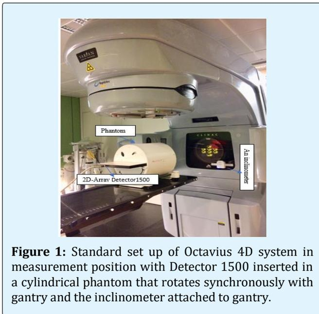
**Figure 1:** Standard set up of Octavius 4D system in measurement position with Detector 1500 inserted in a cylindrical phantom that rotates synchronously with gantry and the inclinometer attached to gantry.
