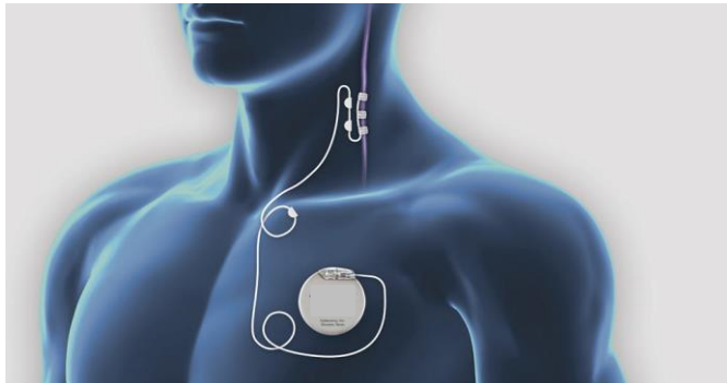
Figure 12. Schematic illustration of the vagus nerve stimulation (VNS) system. The pulse generator is implanted in the subclavicular region and connected to a helical electrode wrapped around the vaugs nerve in the neck through a bipolar lead (adapted from [75]).
