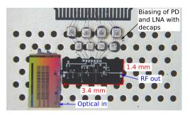
Fig. 7: Narrowband photoreceiver assembly.
