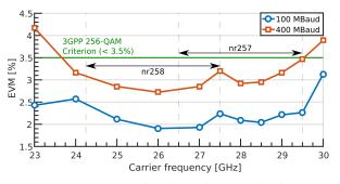
Fig. 12: rms-EVM as a function of the carrier frequency.
