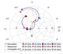
Fig. 9:  $S_{11}$  shown on the Smith chart for a 50  $\Omega$  reference.
