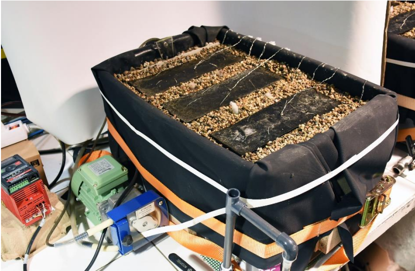
Figure 3.1.2 Photograph of one of the CW-MFC+ systems
