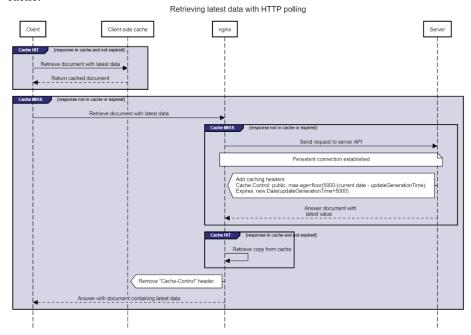
**Fig. 1.** Two cache components (client-side and server-side/nginx) are used for HTTP polling. As Nginx does not dynamically update the max-age value from the Cache-Control header, we fall back on the Expires header for client-side caching.
