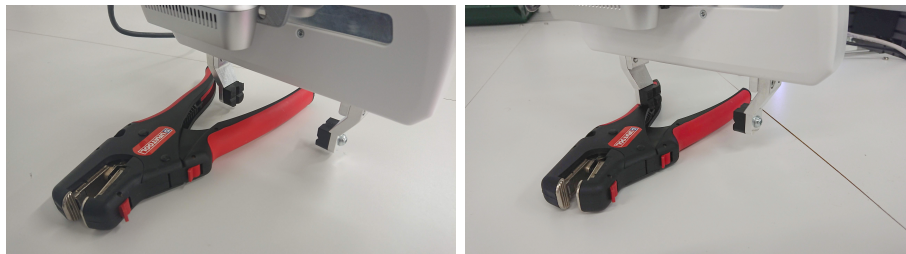
Figure 11: The end-effector’s correct grip position on the left and failed attempt on the right for grasping the wire clipper.
