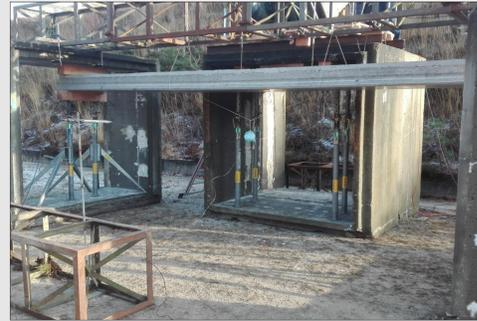
Simply supported hollow core slab
