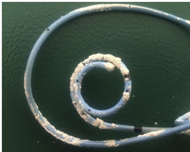
Figure 1 Encrustations on stent surface after 2 weeks indwelling time in chronically infected urinary tract system.
