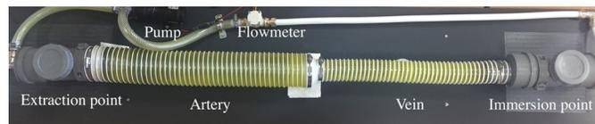
FIGURE 2. Proposed experimental setup to mimic sections of the circulatory system with non-Newtonian fluid (i.e. liquid detergent) flowing in an air-tight circuit.
