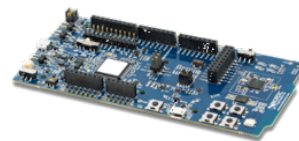
(a) nRF52840 Development Kit from Nordic Semiconductor
