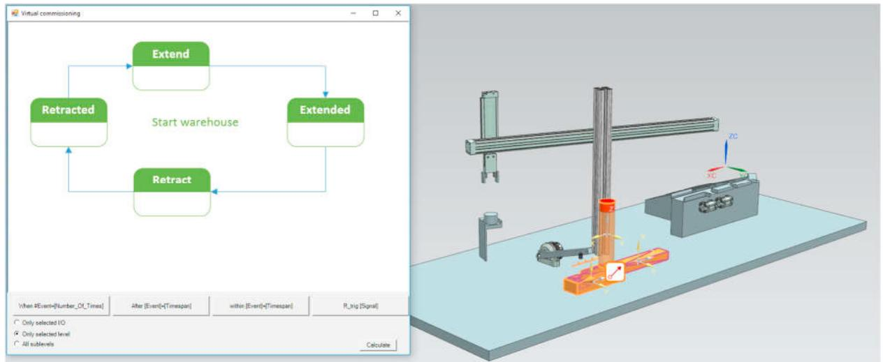
Fig. 2: Defining states and transitions on a subsystem
