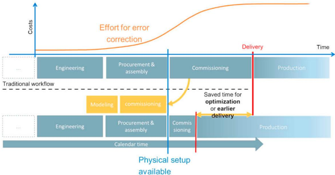
Fig. 1: Automation project timeline and related error correction costs
