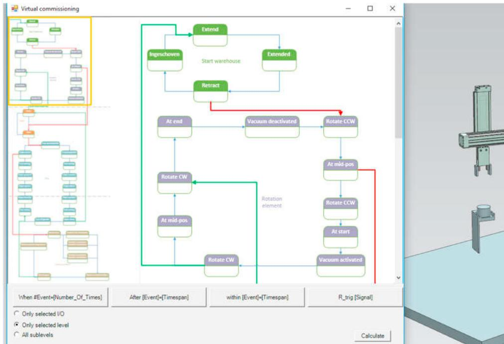
Fig. 3: Defining states and transitions between subprocesses, no subprocess selected
