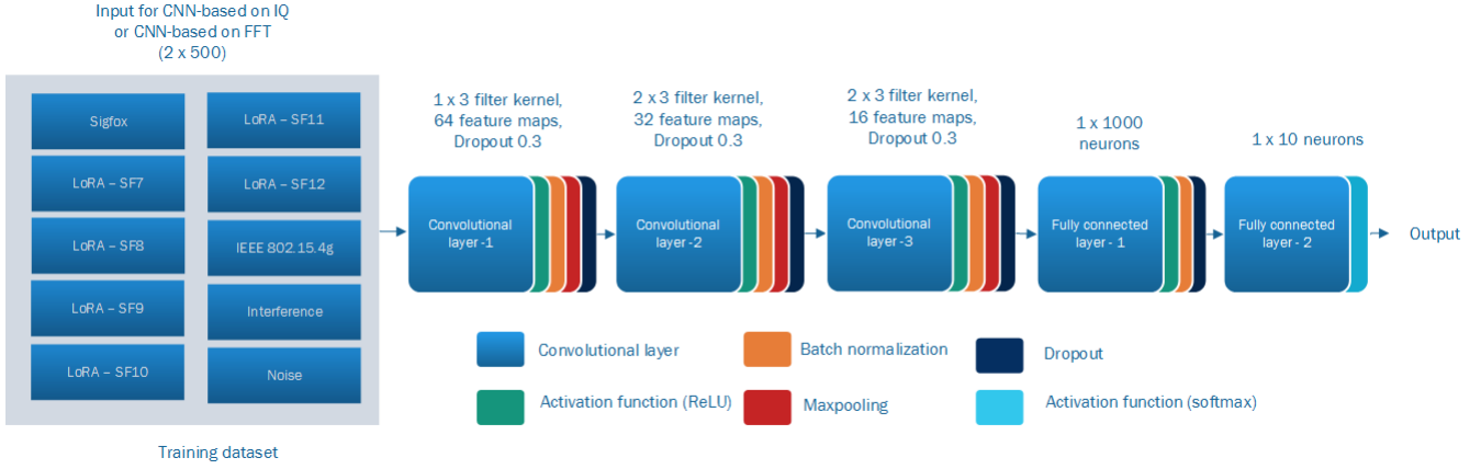
Fig. 5: Proposed architecture for CNN based on IQ and CNN based on FFT.
