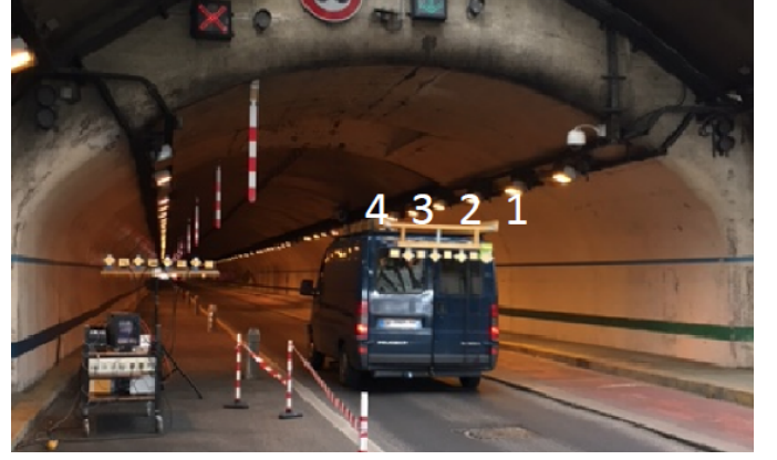
Fig. 1. Cross-section of the tunnel with Tx in the closed lane (left) and Rx in the open lane (right)
